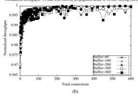
Figure 7. Throughput: varying number of connections compete for the bottleneck link T1 with  $delay=200\ ms$  or  $delay=50\ ms$ .
