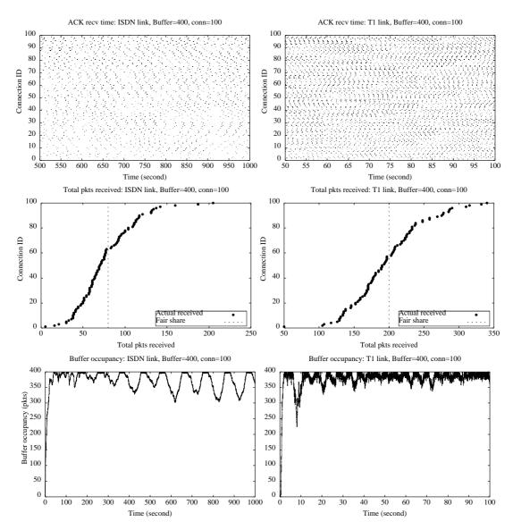
Figure 11. Adding random process time in <u>large pipe case</u> breaks down the global synchronization: 100 connections share the bottleneck link of either ISDN or T1 with one-way propagation delay of 50 ms and bottleneck buffer size of 400 packets. Compared to the case of without random processing time, the buffer occupancy is quite stable. Furthermore global synchronization disappears as shown in the scatter plot for ACK arrival.
