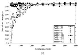
Normalized throughput: T1 link with oneway propagation delay of 50 ms, varying buffer size
