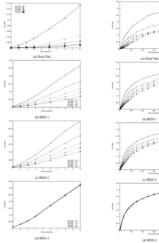
Figure 29. Loss probability for a small number of TCP/SACK connections competing for T1 bottleneck link.
