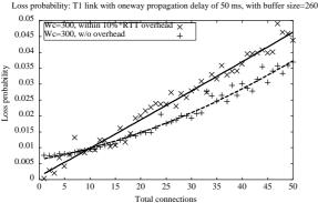
Figure 17. Loss probability for <u>a small number of connections</u> after adding random processing time of up to 10%\*RTT at TCP source: varying number of connections compete for the bottleneck link of T1 link with delay=50~ms. The loss probability grows linearly when the number of connections is small.
