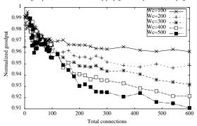
Normalized goodput: T1 link with oneway propagation delay of 50 ms, varying buffer size
