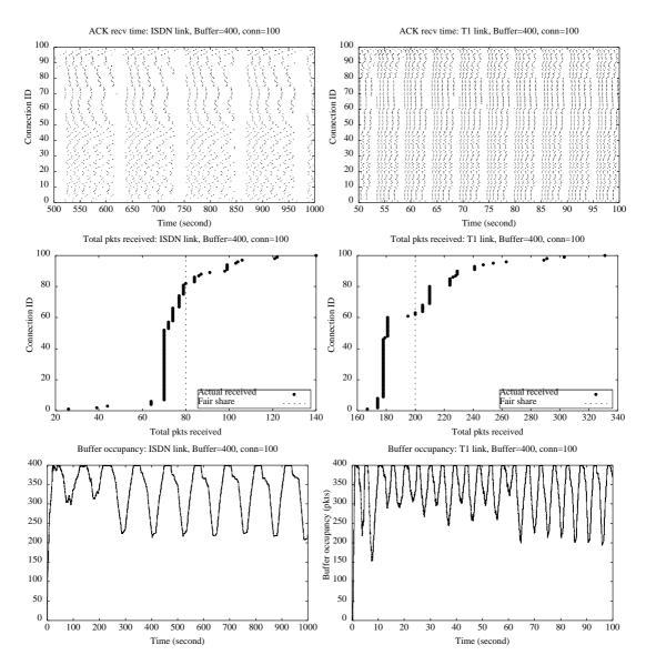
Figure 2. <u>Large pipe case</u> leads to global synchronization: 100 connections sharing the bottleneck link of either ISDN or T1 with one-way propagation delay of 50 ms and bottleneck buffer size of 400 packets. Notice the buffer occupancy fluctuates from half to full periodically. Moreover there are periodic white stripes in the scatter plot of ACK arrival time, where during the white stripes all connections experience loss and try to recover them using fast retransmission.
