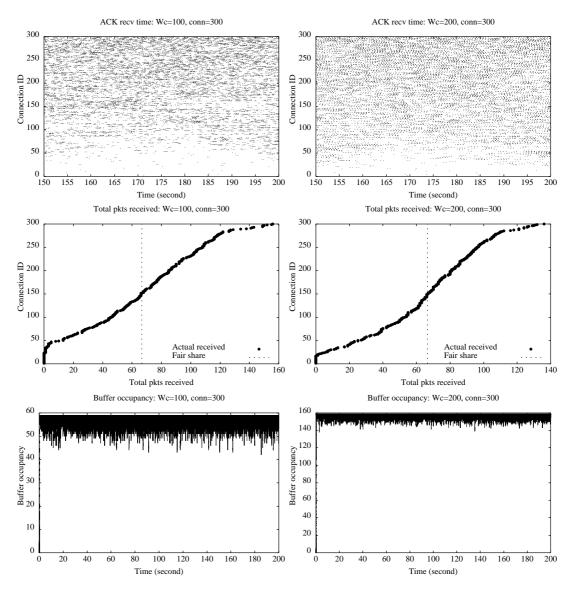
Figure 13. Adding random processing time in small pipe case: 300 concurrent connections compete for T1 link with one-way propagation delay of 50 ms and buffer size of 60 (or 160) packets ( $W_c=W_{opt}+Buffer$ =100 or 200 packets). The buffer occupancy is quite stable, and the consistent discrimination is not as severe as without adding random processing time.
