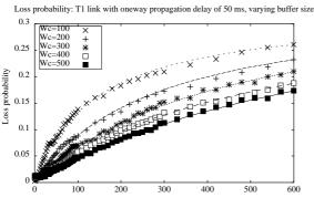
Figure 10. Loss probability for a large number of connections: varying number of connections compete for the bottleneck link of either ISDN or T1. In both cases, propagation delay = 50 ms. The loss probability curves match very well with hyperbolic curves when the number of connections is large, where the parameters of the hyperbolic curves are given in Table 1.
