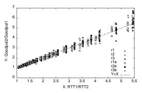
Figure 34. The effect of RED gateway on FTP sessions with 2 different RTT's. The simulation settings are the same as in Fig. 32 except that the bottleneck router uses RED queue management.
