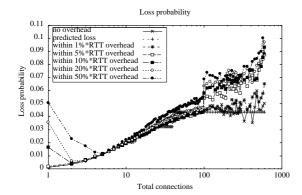
Figure 12. Compare the loss probability by adding different amount of random processing time: varying number of connections compete for T1 link with  $delay=50\ ms$ .
