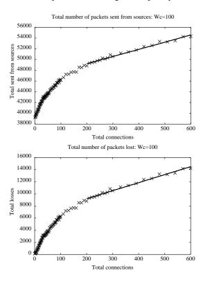
Figure 5. Varying number of connections compete for T1 link with  $delay=50\ ms$  and  $buffer=60\ packets$  ( $W_c=100\ packets$ ): the total number of packets sent and dropped increases linearly with the number of connection when the connection number is large.
