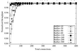
Normalized throughput: T1 link with oneway propagation delay of 50 ms, varying buffer size
