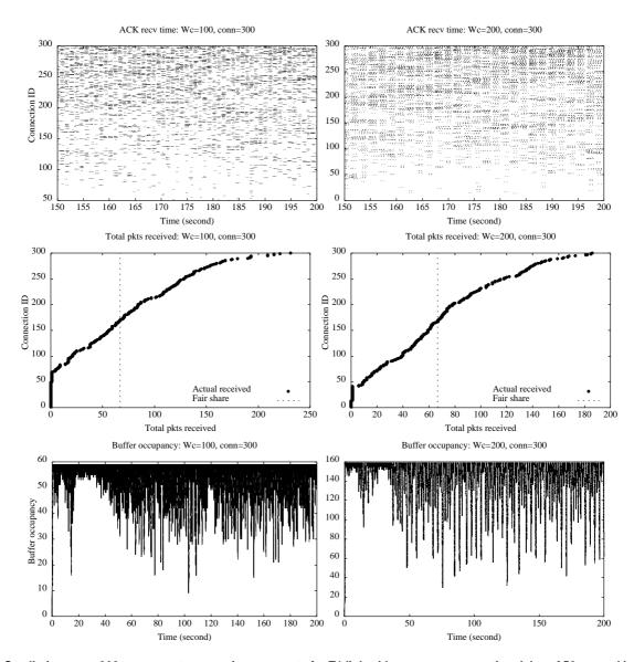
Figure 4. Small pipe case: 300 concurrent connections compete for T1 link with one-way propagation delay of 50 ms and bottleneck buffer size of 60 (or 160) packets ( $W_c=W_{opt}+Buffer=$  100 or 200 packets). Note that the buffer occupancy fluctuates widely. Moreover part of connections receive little goodput as shown in the two graphs in the middle.
