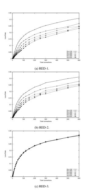
Figure 26. Loss probability for a large number of connections competing for T1 bottleneck link with RED.
