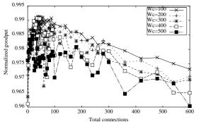
Figure 8. Goodput: varying number of connections compete for the bottleneck link of either ISDN or T1. In both cases,  $delay=50\ ms.$
