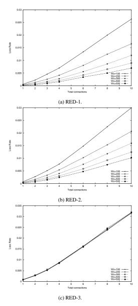
Figure 25. Loss probability for a small number of connections competing for T1 bottleneck link with RED.
