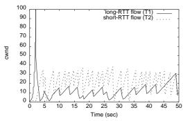
Figure 33. The congestion window evolution of two TCP flows  $T_1$  and  $T_2$  with Drop-Tail FIFO queue management.  $RTT_1>RTT_2.$
