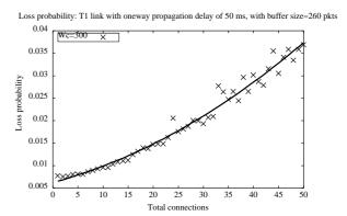
Figure 9. Loss probability for <u>a small number of connections</u>: varying number of connections compete for the bottleneck link of T1 with  $delay=50\,ms$ . The loss probability grows quadratically when the number of connections is small.
