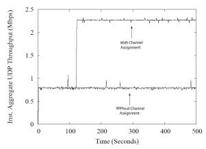
(a) Instantaneous aggregate client throughput on Linear topology. Improvement seen is a result of channel assignment.
