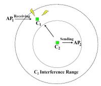
Figure 6: Illustration of *two-hop* interference scenario.  $C_2$ 's data packets collide with data packets being received by  $C_1$ .  $AP_1$  and  $AP_2$  interference ranges have been elided for clarity.
