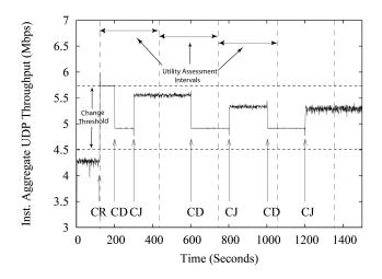
Figure 16: Instantaneous aggregate client throughput in smallscale scenario. Following events are shown: CR=Configuration Re-computation, CJ=Client Join, and CD=Client Disconnect. Utility assessment intervals shown as vertical dotted lines and change threshold shown as horizontal dotted lines.
