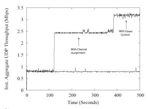
(b) Instantaneous aggregate client throughput on Star topology. Initial improvement is because of channel assignment while the subsequent improvement comes as a result of power control.
