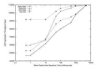
Figure 3: Throughput obtained by a node in the presence of interference. The x-axis indicates the mean delay between successive packets sent by the interferer (see Figure 2)
