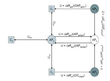
Figure 4: Annotated Conflict Graph. Circular vertices are access points and square vertices are clients. Basic conflict graph (used for channel assignment) contains only the circular vertices, shown in the figure. Clients have the same channel as their associated access point.
