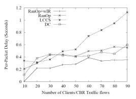
Figure 14: Per-packet delay at 30dbm using 3 channels
