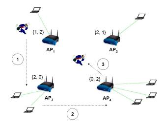
Figure 15: Micro-benchmark setup for analyzing impact of mobility. User mobility shown as dotted arrows with labels indicating steps followed by client. For large-scale scenario, channels are shown in curly brackets where the numbers depict assignments before and after large-scale change.
