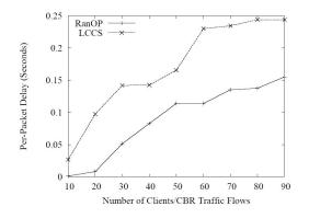
Figure 13: Per-packet delay at 30dbm using 12 channels
