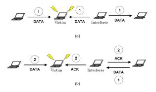
Figure 2: (a) illustrates a Data-Data collision scenario where *victim* is the node experiencing interference. (b) illustrates a Data-Ack collision scenario wherein the direction of traffic flow at the *interferer* is reversed. The steps that occur in each scenario are labeled accordingly.
