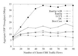
Figure 12: Aggregate client throughput at 30dbm using 3 channels
