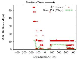
Figure 6: Example of poor rate selection using the default parameters of the default bit rate selection algorithm. Using these parameters would have resulted in 75% less overall throughput compared to using our modified parameters which achieved much higher rates (shown in Figure 5(b)). The lack of throughput during the middle of this run was due to a TCP timeout, caused by an initially excessive bit rate of 54 Mbps.
