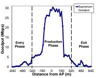
Figure 11: The three phases of a vehicular connection
