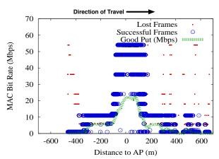
Figure 17: Example of overestimation of initial MAC bit rate; 54 Mbps was chosen although only 1 Mbps was possible during the initial phase of the connection. In this run it took 115 m (6 s) to adapt to the proper bit rate. Also seen later in the connection are the frames used to probe higher rates.
