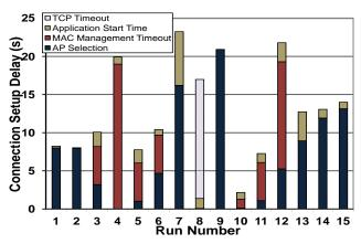
Figure 14: Cumulative bar graph showing the breakdown of the sources of delay for 15 runs
