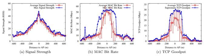
Figure 5: Measured signal strength (RSSI), MAC bit rate, and goodput averaged over distance across 15 runs with 95% confidence intervals. The maximum potential connection spans a distance of 1280 m which lasted 58 seconds at a speed of 80 km/h.
