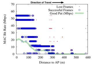
Figure 21: Example run showing overestimation of MAC bit rate after production phase causing a TCP timeout at 300 m (last half of connection shown).
