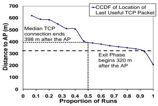
Figure 22: CCDF showing the location where the TCP connection became un-usable. As shown, the majority of runs ended early into the exit phase.
