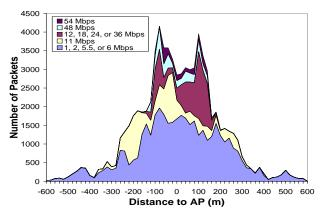
Figure 19: Breakdown of MAC bit rates used by the vehicular client for sending TCP ACKs, aggregated across 15 runs. The unusual two peaks in the curve are explained in Section 6.3.2.
