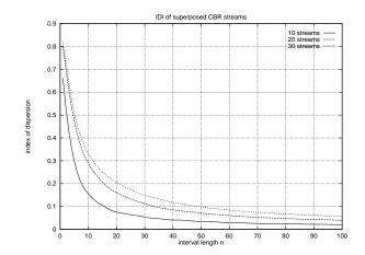
Figure 6: The IDI for the superposition of a number of CBR streams with arbitrary bandwidths.
