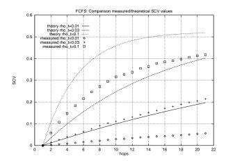
Figure 20: Comparison of analytic and measured SCV as a function of number of hops for different tagged stream intensities  $\rho_T$ .
