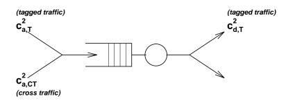
Figure 18: The model used to approximate one segment in the multihop topology.
