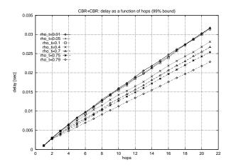
Figure 7: The end-to-end delay in function of the number of hops the cell goes through (FCFS).
