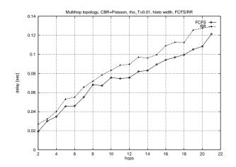
Figure 15: The delay histogram width as a function of the number of hops the tagged stream goes through, with  $\rho_T = 0.01$ .
