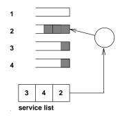
Figure 2: A RR/WRR implementation using service lists is considered. This approach is preferable from a hardware point of view, as no "search" operations need to be performed to find the next connection requiring service.
