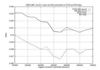
Figure 8: The end-to-end delays (mean and 99%-percentile) for FCFS and RR scheduling for different bandwidth partitions. The total link utilization  $\rho$  was kept constant at 0.9. The values shown are ensemble averages over phase combinations.
