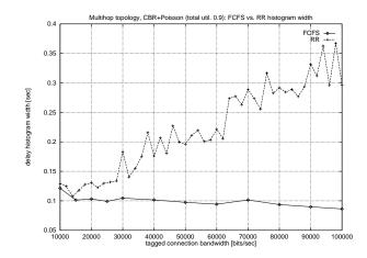
Figure 13: The histogram width of the measured end-to-end delay after going through 21 switches for FCFS and RR.
