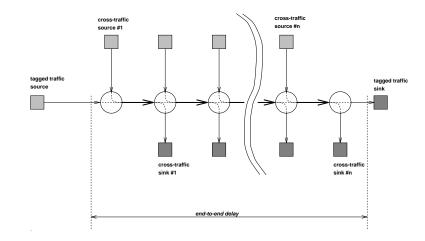
Figure 3: The *multihop* topology used to simulate the interactions with other streams and the resulting impact on the characteristics of a "tagged" connection.
