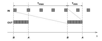
Figure 16: Incoming cells experience different delays, ranging from  $T_{min}$  to  $T_{max}$ , depending on when they arrive within a round. Service of the considered connection begins at **B**, and service of all other connections begins at **A**.
