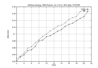
Figure 14: The 99%-delay-percentile as a function of the number of hops the tagged stream goes through, with  $\rho_T = 0.01$ .
