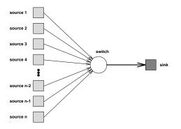
Figure 4: The topology used to study the characteristics of a CBR superposition process.
