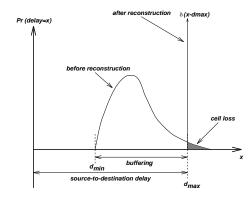
Figure 1: The relationship between the end-to-end delay histogram measured *before* the reconstruction buffer, and how buffering and delay *after* the reconstruction buffer can be determined.
