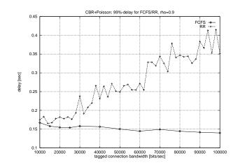
Figure 12: The 99%-percentile of the measured end-to-end delay after going through 21 switches for FCFS and RR.
