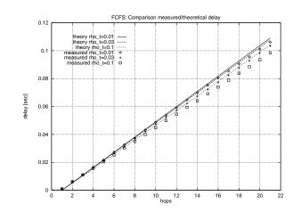
Figure 21: Comparison of analytic and measured delay as a function of number of hops for different tagged stream intensities  $\rho_T$ .
