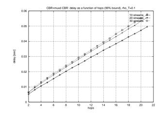
Figure 9: The end-to-end delay as a function of the number of hops (FCFS).
