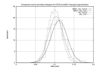
Figure 17: Two end-to-end delay histograms and the delay distribution resulting from the M/D/1-Gaussian approximation
