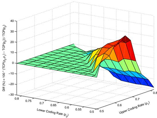
(a)  $p_e = 10^{-2}$ . % Deviation of Single-Rate model with parameters  $(C_0, p_0, R_0)$ .
