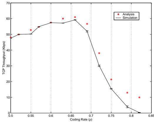
Figure 6: *Single-Rate case*: TCP throughput for a bit error probability of  $p_e = 10^{-2}$ .
