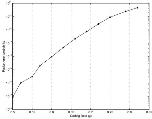
Figure 5: Packet error probability  $p$  as a function of the coding rate  $\rho$  for a bit error probability of  $p_e = 10^{-2}$ .
