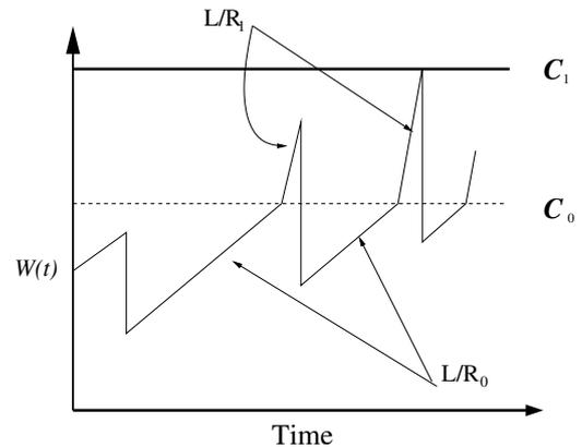
**Figure 2: TCP window size evolution over a variable rate channel.**
