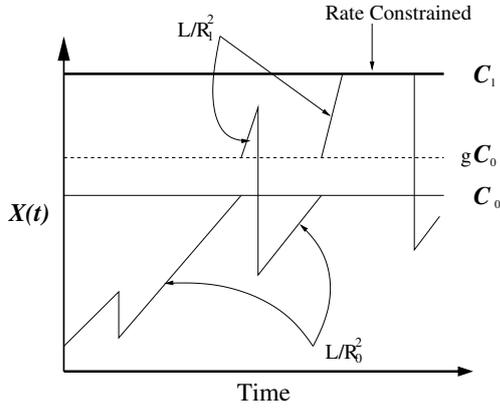
**Figure 4: TCP Evolution when maximum advertised window  $W_{max} = C_1 \cdot R_1$ .**
