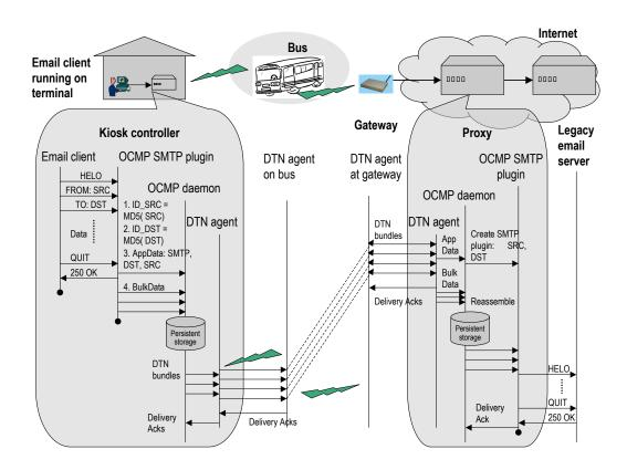
Figure 3: KioskNet data path when used to send email from a kiosk to the Internet.
