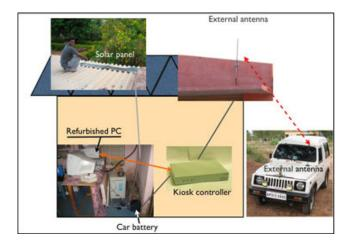
Figure 5: Composite picture of the pilot deployment.
