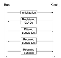
Figure 4: Meta Data Exchange Protocol.
